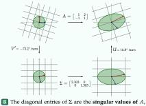
and the columns of U and V are called left singular vectors and right singular vectors, respectively. A maps each right singular vector  $\mathbf{v}_i$  to the corresponding left singular vector  $\mathbf{u}_i$  scaled by  $\sigma_i$ .
